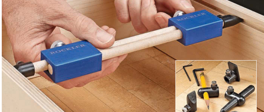
▲ Bar gauges can go where tape measures can't. Here, the tapered tips of the gauge fit inside the grooves on a drawer to size the bottom panel.
