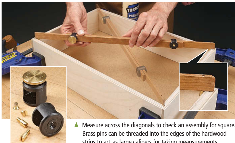
▲ Bar gauges can go where tape measures can't. Here, the tapered tips of the gauge fit inside the grooves on a drawer to size the bottom panel.
