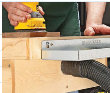
▲ A dust port on the side of the benchtop allows it to function as a downdraft sanding table.
