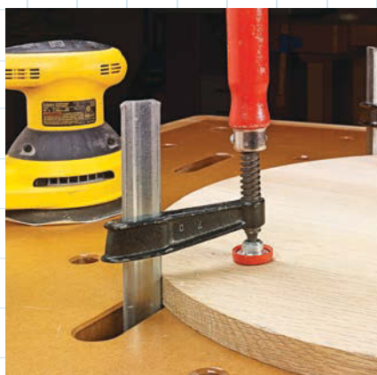
▲ Holes and slots in the benchtop allow you to conveniently clamp a workpiece in place.
