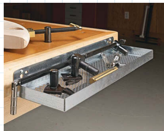
▲ A wire mesh auxiliary tray keeps often-used items close at hand without collecting sawdust.
